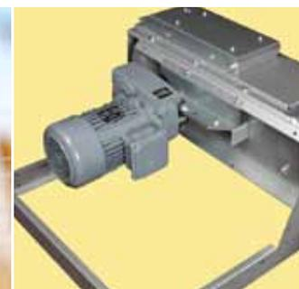
Direct-mounted gearbox motor with support frame.
